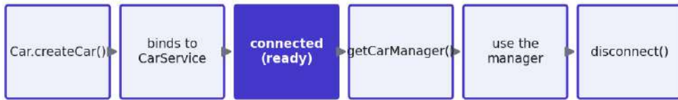
An app connects to CarService, gets the manager it needs, then disconnects when done
